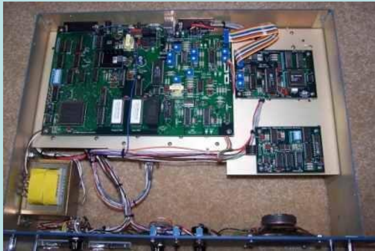
CAT-1000 Controller, Digital Voice Recorder, and Audio Delay Board
