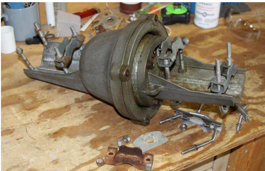
Bottom view 4-wire rotor system (No Brake. No potentiometer position feedback)
